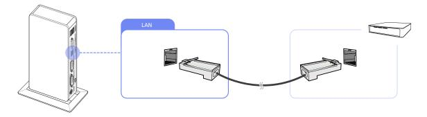
1 Connect the LAN cable to the [LAN] port at the back of the product.
